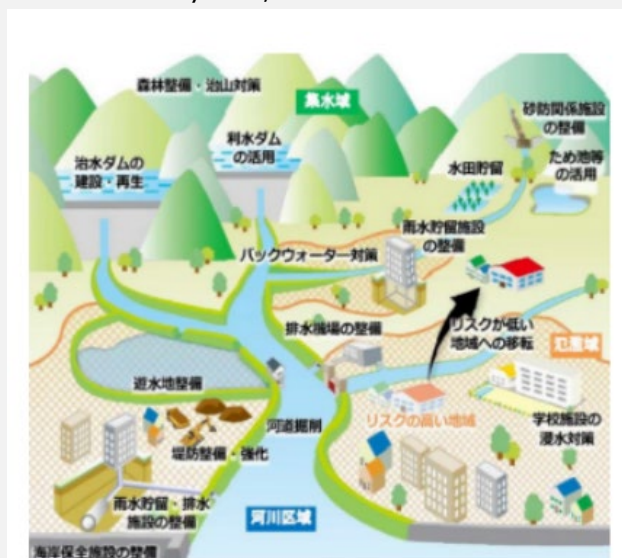
Figure 2: Conceptual Diagram of River Basin Disaster Resilience and Sustainability by All Source: Ministry of Land, Infrastructure, Transport and Tourism
